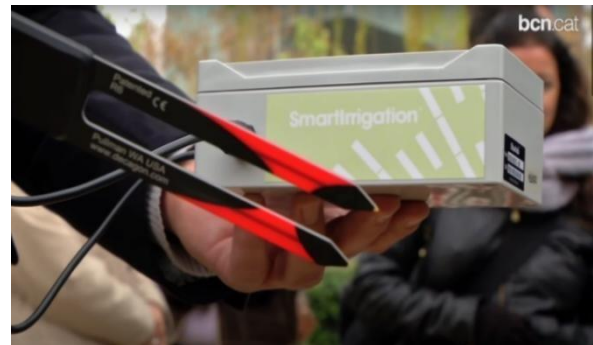
Figure 2 Smart irrigation unit with water level sensor in Barcelona (source: ajuntament.barcelona.cat)
