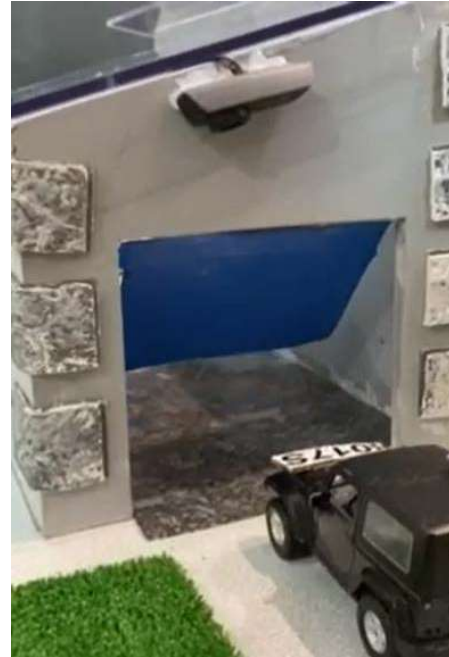
Figure 1 The webcam recognizes the license plate and opens the garage door
