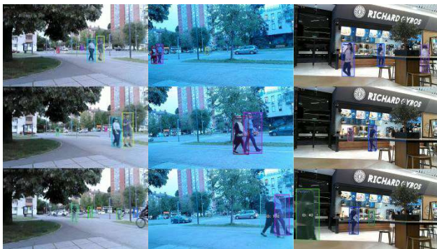
Figure 2 (a) succesful ReID, but with low fps rate due to dynamic background noise; (b) succesful ReID under low light conditions, but with identity loss after change of person's orientation at the end of sequence; (c) retail store application.
