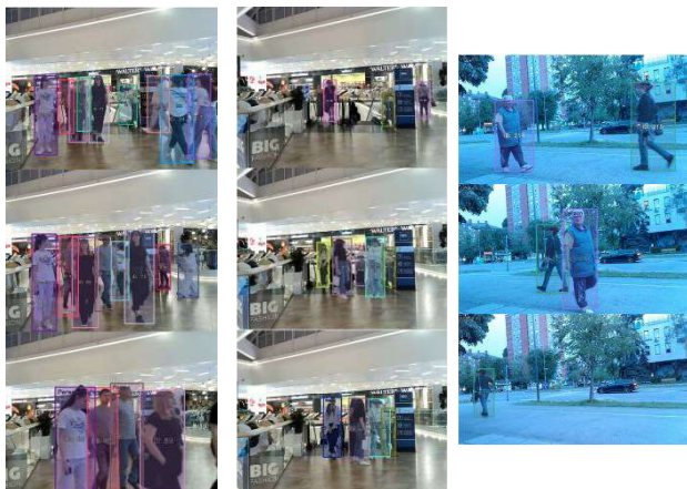
Figure 3 (a) crowded indoor space: succesful ReID, but with low fps; (b)~false person detection, but with correct ReID; (c)~low light operation.
