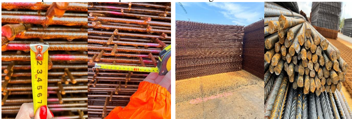
Figure 4-Product control, the quality of the finished products - reinforcing mesh and ribbed reinforcing bars - was checked on the spot.
